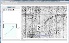
A suite of data visualisation tools for viewing high resolution seismic data, 3D digital terrain models (DTM) and borehole logs.
